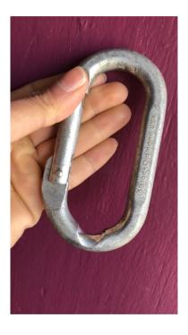
Metal components should be replaced if more than 10 percent of the metal has been worn away. Components made of fabrics, such as slings, are also susceptible to wear and should be inspected regularly and replaced if there is significant wear.
