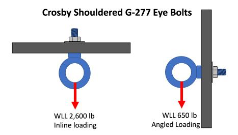
As you can see, the specified WLLs are considerably different, based on how the hardware is loaded. If you do not know how the angle of the force on the hardware you are use affects its WLL, then your aerial point may not be as strong as you believe it is.
