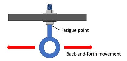
It could take months or years, but the metal will fatigue over time. The longer the shaft, the greater the level, the greater the force at the stress point, and the faster fatigue occurs. For this reason, shouldered eyebolts are recommended for many aerial points.
