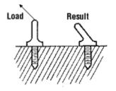
The load must be "in-line" with the axis of the eye, not perpendicular.
