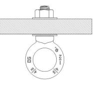
A ½" diameter eye bolt has a Working Load Limit (WLL) of about 2,600 lbs. with a 5:1 safety factor, giving a breaking strength of about 13,000 lbs. This is well over our design goal of 5,000 lbs.
